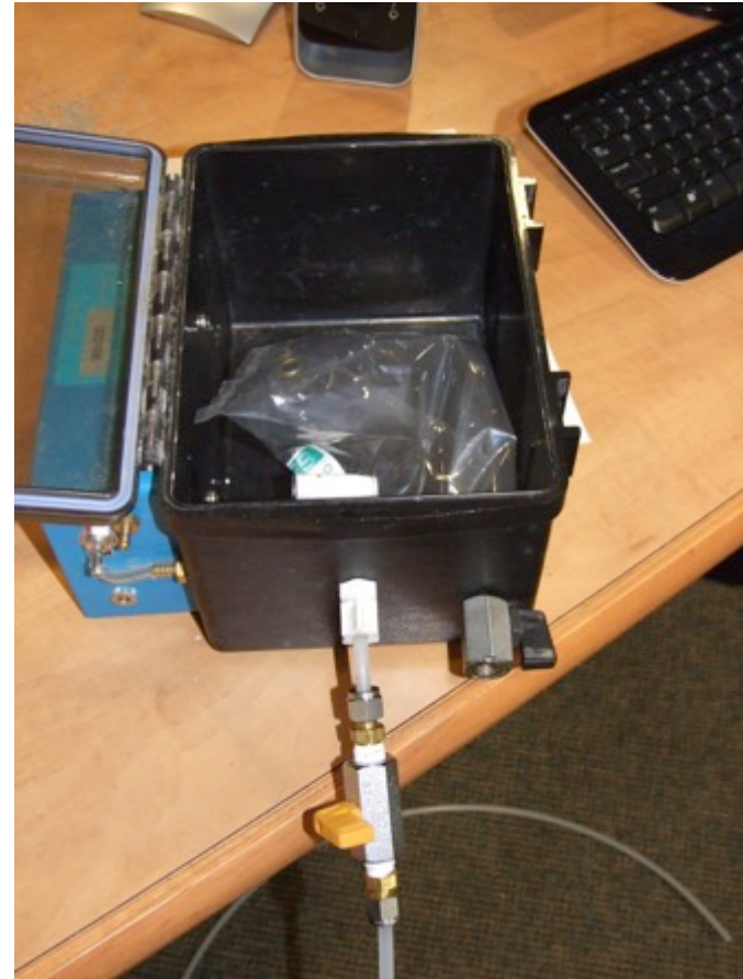
Lung box – Tedlar bag sample (Handheld monitor – helium, gases & VOCs)
